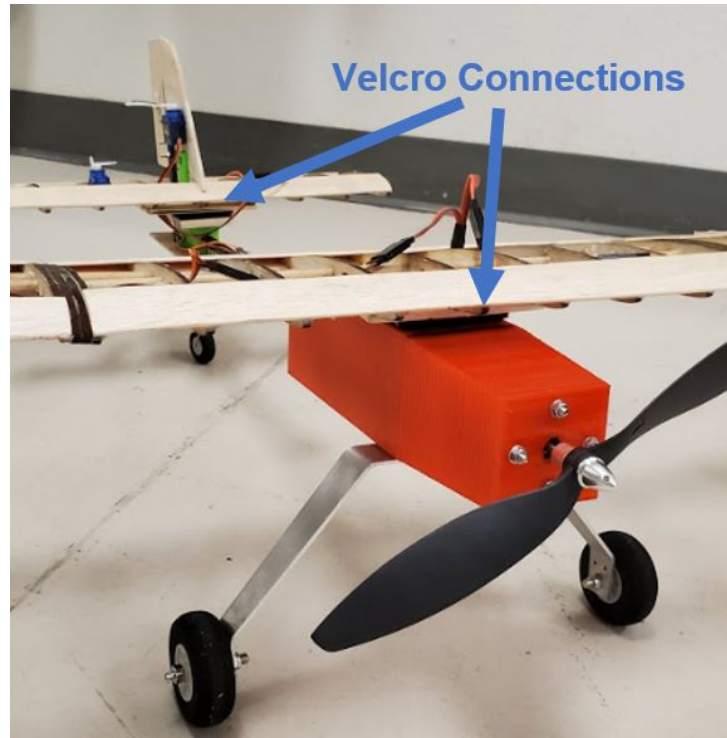
Figure 15: Velcro Wing Connections
