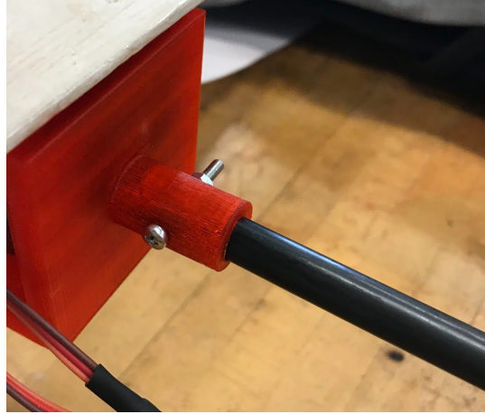
Figure 6: Carbon fiber rod connected to fuselage
